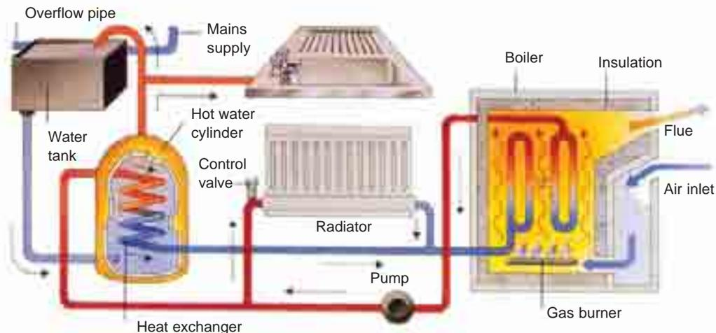
In this central heating system, a furnace burns fuel to heat water in a boiler. A pump forces the hot water through pipes that connect to radiators in each room. Water from the boiler also heats the hot water cylinder. Cooled water returns to the boiler.
