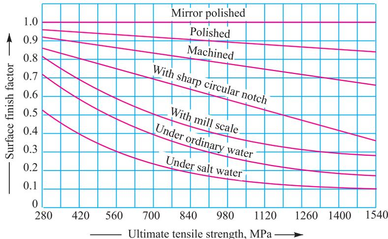
Fig. 6.3. Surface finish factor for various surface conditions.
