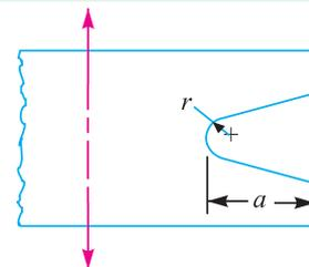
Fig. 6.7. Stress concentration due to notches.
